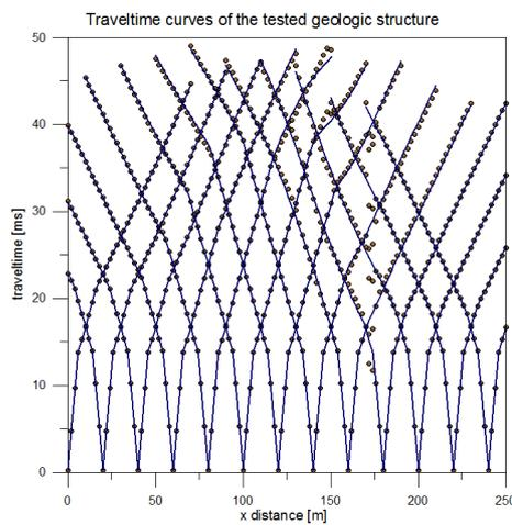
**Figure 1** Comparison of the traveltimes curves of the initial and calculated geologic structures
