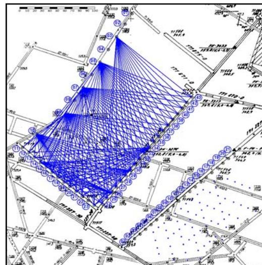
Figure 2. Map of the geoelectric seam-soundings and transillumination measurement system.
