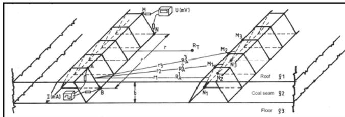
Figure 1. The scheme of seam-soundings and seam-transillumination.
