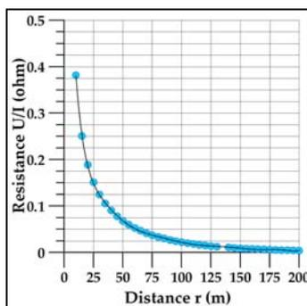
Figure 6. Apparent resistance  $R^{(0)}$  master curve for tomography, calculated from model in Table 1.
