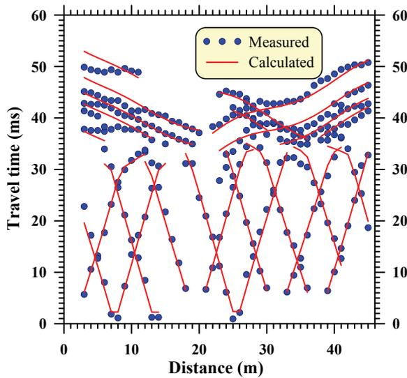
Figure 2a: Measured and calculated first breaks for P-waves
