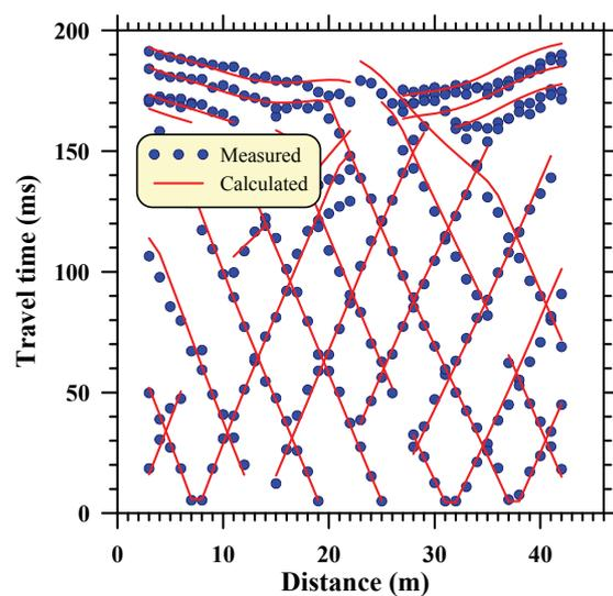
Figure 2b: Measured and calculated first breaks for SH-waves
