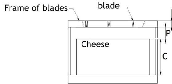
Figure 3. The cutting chamber with the cheese
