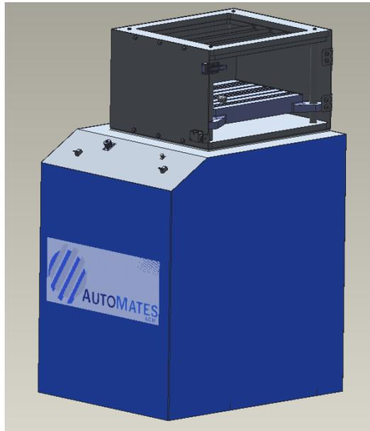
*Figure 11. The Model of the cheese cutter machine*
