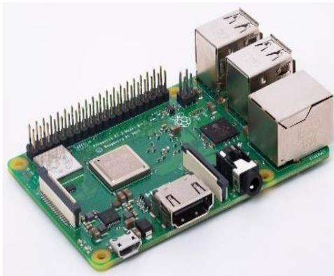
Figure 16. Raspberry Pi 3 Model B+
