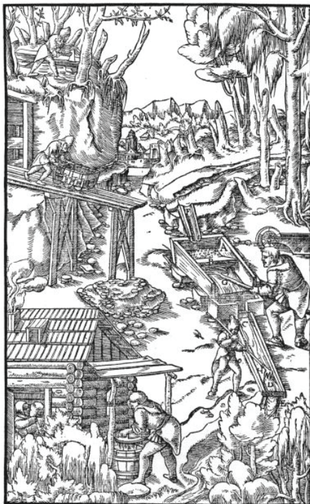
A—BOX. B—PERFORATED PLATE. C—TROUGH. D—CROSS-BOARDS. E—POOL. F—LAUNDER. G—SHOVEL. H—RAKE.
