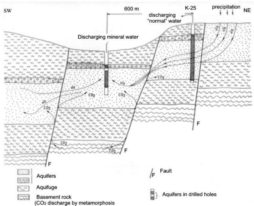
Figure 1. Hydrogeological profile of two boreholes. where the downflow and upflow zones were observed (Edited by P. Prakfalvi P. drawn by J. Kakuk)
