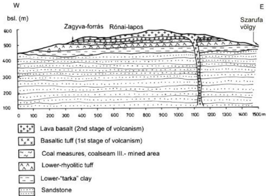
Figure 2. Distribution of basalt rock on the surface is incomparably greater than the area of horizontal section of volcanic breakthroughs
