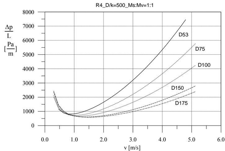
Figure 1. Calculated pressure loss curves ( $\Delta p/L - v$ ) of fly ash–slag water mixtures of the Mátra Power Plant. Parameter: pipe diameter. (Research report 1998.)
