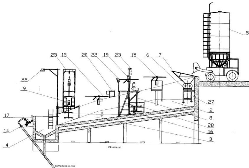
2 - first mixing pool, 3 - second mixing pool, 4 - last pool with pipeline input, 5 - lime silos, 6 - 27 - fly ash breaker, 7 - sieve, 8 - 9 - 28 - mixer, 14 - 17 - washing water valve, 15 - 19 - water jets, 16 - slurry pumps
