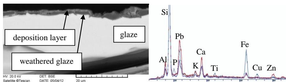
Figure 6. Cross-section of a glazed ceramic tile: the upper light grey deposition layer and the dark grey weathered glaze beneath covering the unaltered glaze (on the left). In the bottom-right corner of the BSE image a 10 µm wide crack is located in the glaze. X-ray spectra show the chemical composition of the deposition layer (grey), the weathered glaze (blue) and the unaltered glaze (red) (on the right)
