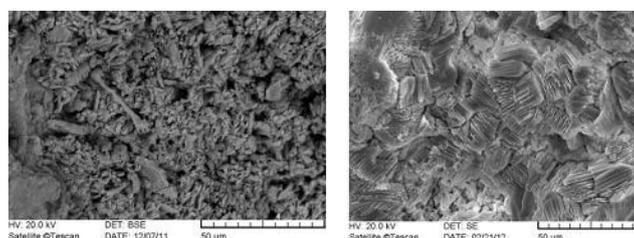
*Figure 4. Dense, compact gypsum layer (on the left, BSE image) and laminar gypsum layer (on the right, SE image) on the unglazed, back side of the ceramics*
