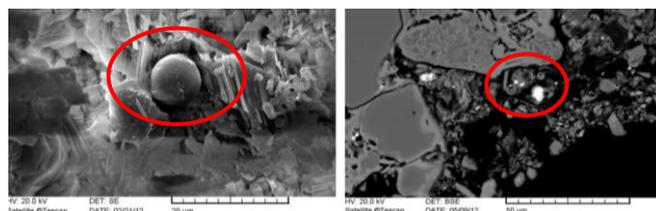
*Figure 3. Scanning electron microscope pictures of natural and artificial spherules. 20 µm wide natural spherule with complex composition (Si, Fe, Ca, Al rich) in compact gypsum crust on the glazed side of a ceramic tile (on the left) (SE image) and a bright Fe-rich and several dark, carbonaceous artificial, 5-15 µm sized (in diameters) spherules in the dust layer on the unglazed (back) side of a ceramic tile (on the right) (BSE image)*
