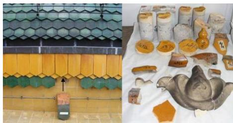
Figure 2. A green glazed tile from the roof of the the Museum of Applied Arts (on the left) and the studied samples of pyrogranite elements (on the right)
