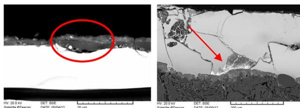
Figure 7. The weathered surface layer of glaze is fragmented (on the left) and the weathered glaze with bright precipitations rich in lead occurs along the cracks and at the ceramic-glaze interface (on the right) (BSE images)
