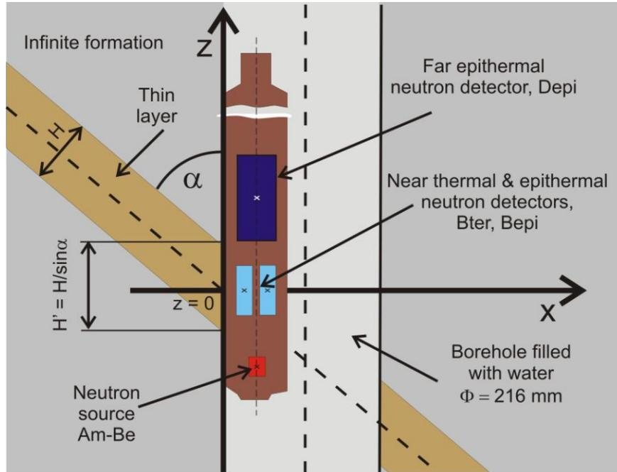
Figure 1. Formation – borehole geometry for MC modeling.
