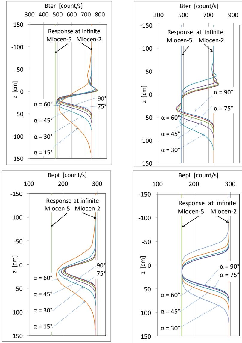
Figure 2. Neutron profiles modeled by *m-c* simulations for *Bter* and *Bepi* detectors for different slope angles,  $\alpha$ , for *Miocen-5* thin layer: left:  $H = 15$  cm, right:  $H = 50$  cm thickness. The layer is surrounded by *Miocen-2* rock model. Description of the  $z$  axis - as in Fig. 1.
