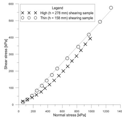
Figure 4. Effect of sample height reduction on Coulomb failure lines during shear tests
