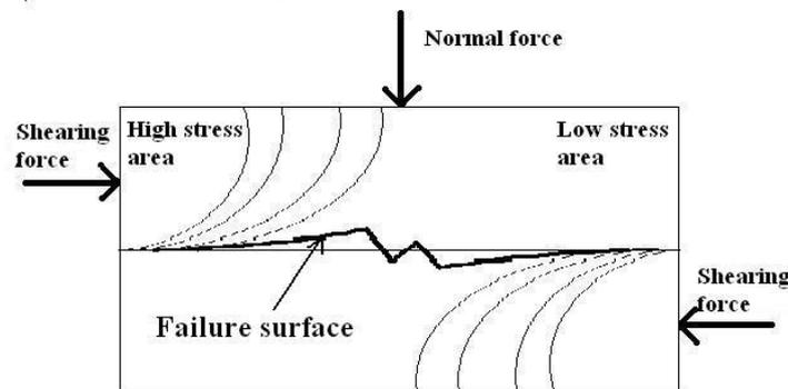
Figure 6. Stress distribution in a shear sample (reconstruction by authors)
