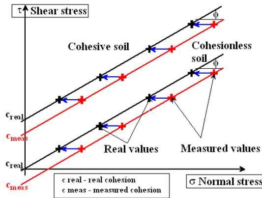
Figure 3. Theory of effect of friction on wall to the cohesion
