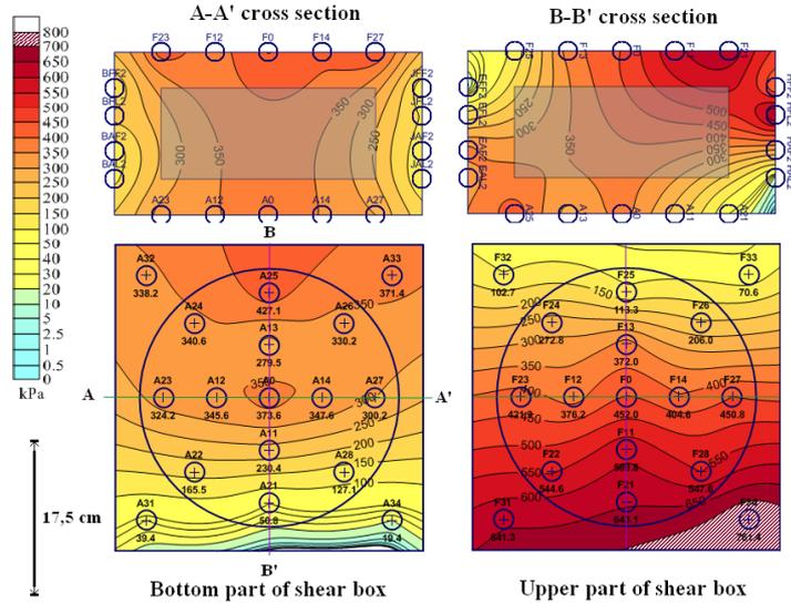
Figure 7. Stress distribution in large scale shear sample (pressure sensors)
