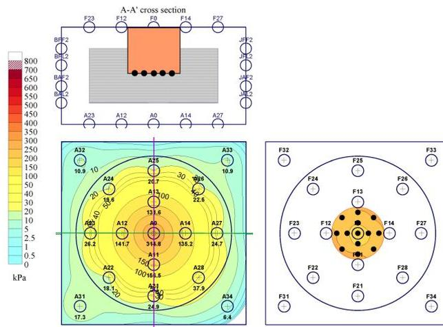
Figure 8. Stress distribution in an indenter test (pressure sensors)
