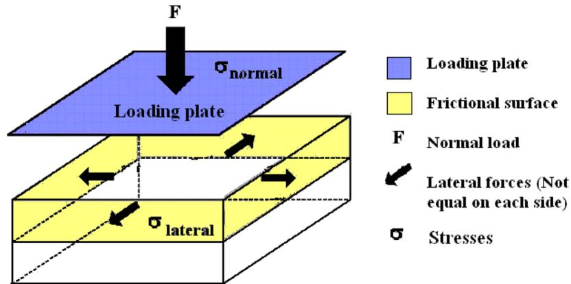
Figure 2. Scheme of surfaces and stresses causing side wall friction
