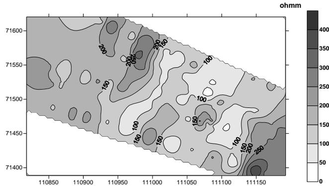
Figure 1. VLF apparent resistivity map due to GBR at Köpüs Spring
