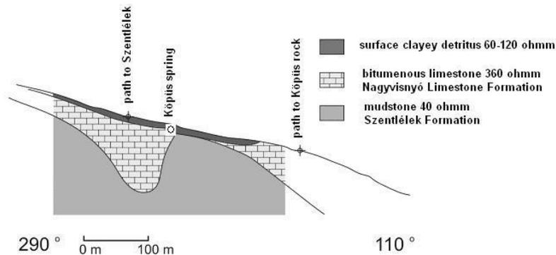
Figure 3. Interpretation based on resistivity and phase at Köpüs Spring
