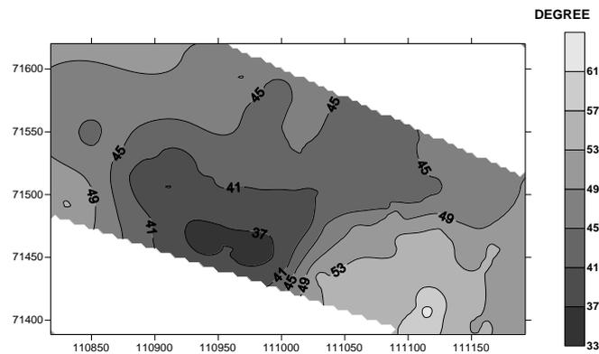
Figure 2. VLF apparent resistivity phase map due to GBR at Köpüs Spring
