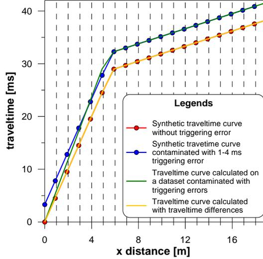
Figure 1. The representation of the evaluation problems of triggering errors in the traveltime dataset
