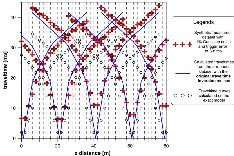
Figure 2. Results of the normal traveltime inversion method:  $D=40.1\%$  (data misfit) from the measured erroneous dataset, and  $d=28.5\%$  (model misfit) from the exact model.
