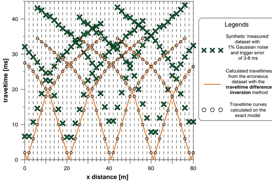
Figure 3. Results of the traveltimes difference inversion method: data misfit of  $D=5.1\%$  from the measured erroneous dataset and a model misfit of  $1.0\%$  from the exact model.
