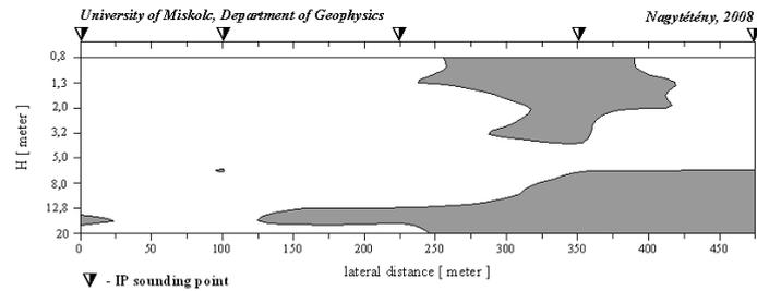
Figure 4. Vertical section of membrane effect ( $0.2 \text{ sec} < \tau < 0.8 \text{ sec}$ )
