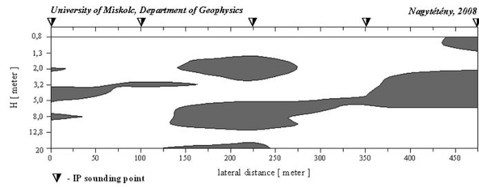
Figure 2. Vertical section of metallic effect ( $1 \text{ sec} < \tau$ )
