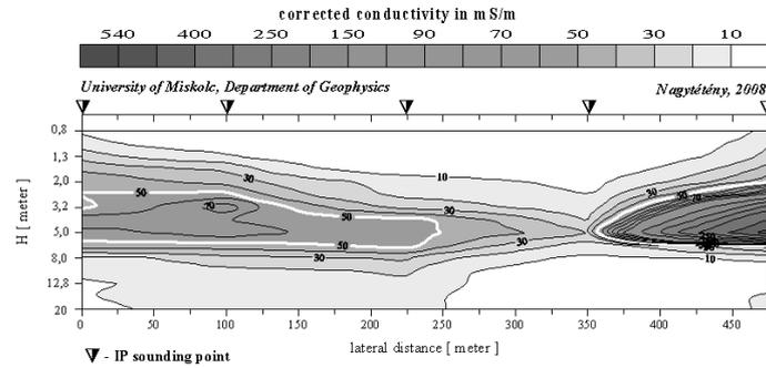
Figure 5. Vertical section of the corrected apparent conductivity
