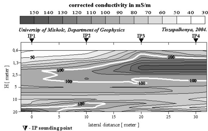
Figure 8. Vertical section of the corrected apparent conductivity
