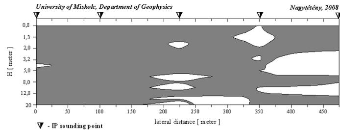
Figure 3. Vertical section of redox effect ( $0.6 \text{ sec} < \tau < 1.2 \text{ sec}$ )
