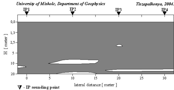
Figure 7. Vertical section of redox effect ( $0.6 \text{ sec} < \tau < 1.2 \text{ sec}$ )
