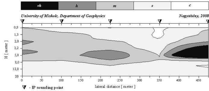
Figure 1. Vertical WAV section (WAV levels:  $> 0.2$  – very high;  $0.1-0.2$  – high;  $0.05-0.1$  – medium;  $0.02-0.05$  – small;  $< 0.02$  – clean)
