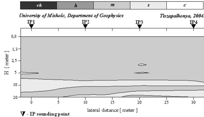
Figure 6. Vertical WAV section at Tiszapalkonya (WAV levels:  $> 0.2$  – very high;  $0.1-0.2$  – high;  $0.05-0.1$  – medium;  $0.02-0.05$  – small;  $< 0.02$  – clean)
