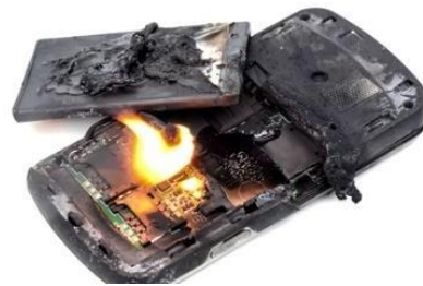
Figure 3: Li-ion failure in a smartphone
