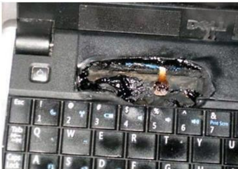
Figure 2: Li-ion failure in a laptop
